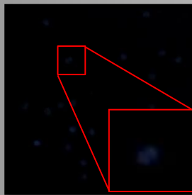
Fig. 5: Too dark. Increasing exposure time or gain may help. Or modify staining protocol. Only the brightest objects are visible.
