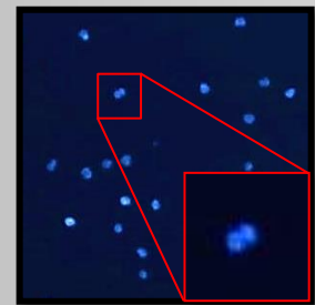
Fig. 7: Ideal illumination, staining and focal plane. No high background, most of the objects have an intensity around 130 grey-scale, objects are sharp and rich in contrast.
